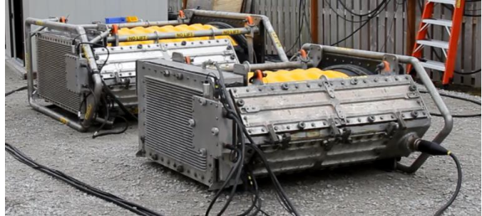
Figure 3: (Left) Contiguous amplitude spectra for the Subtone and Triton flexensional marine vibrator units. Note the two resonance frequencies ('A' and 'B') for each spectrum; (Right) MV units ready for testing.
